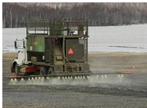
Spattering fluid dust control agent by truck for stabilizing mining tailings
